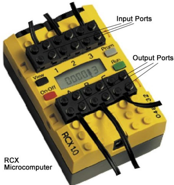
Figure [1]: The RCX™ Microcomputer [2]
